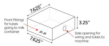
Under-the-Counter Fridge must be professionally modified to include a 2.5" access hole on the top or side of the fridge for milk tubes and wiring connecting the machine to the Milk Pump Unit inside the fridge. It must be within 4 feet of the espresso machine.
