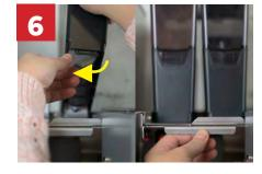
Make sure the dispensers are towards the middle into the mixer unit. Right powder hopper dispenser should be to the left. Left powder be to the left. Left powder hopper dispenser should be to the right.
