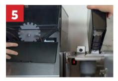
Insert back the container to the base. Refill the powder hopper with powdered drinks.
