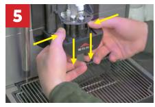
Push the tabs on the brewing spout assembly in and down to disconnect it from the machine.
