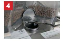
Insert 1 Egro Coffee Machine Cleaning tablet into the chute on the top of the machine. Continue following on-screen instructions.
