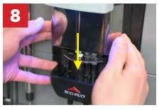
Slide the silver outlet cover down. The cleaning has been completed.
