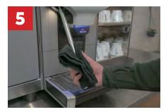
Remove the steam wand from the clean water. Wipe down the steam wand and activate the purge function. The steam wand is now ready for use.
