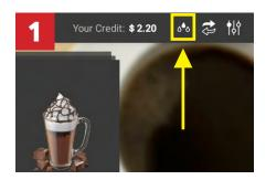
On the upper right corner of main screen, tap on the water drop icon to enter the Cleaning Menu.
