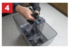
Remove the lids and empty both halves of the bean hopper. Wipe clean with a dry cloth. If necessary, the bean hoppers can be cleaned with soap and water or in a dishwasher.
