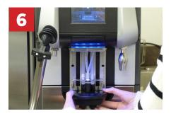
Reassemble brew head. Insert back brew head into the machine, pushing firmly up to lock into place.
