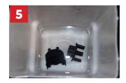
Separate both pieces of the brew head and place into the solution. Allow to soak for at least 1 hour
