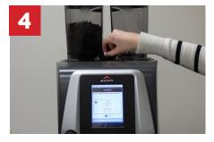
Insert cleaning tablet into the chute on top of the machine.
