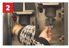
Press the power button to switch off the powder module. Pull out the tube connected to the mixer.
