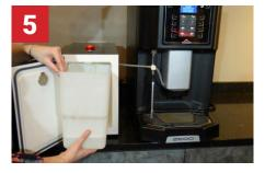
Place the container in the milk storage refrigerator, insert the milk line into the solution, and press "Enter".
