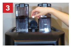
Place an Egro Coffee Machine Cleaning Tablet in the chute on top of the machine.
