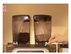
If installed, use key to unlock hopper lid. To disconnect the bean hopper, pull the metal lock located in front of the bean hopper until it clicks.
