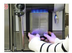
Slide silver cover of coffee outlet down to finish brewing head cleaning.
