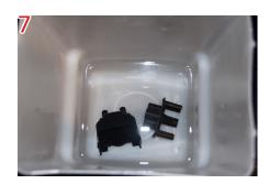
Separate both pieces of brewing head and place into the solution. Allow to soak for at least 1 hour.
