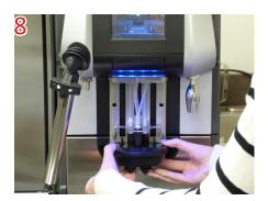
Reassemble brewing head and insert back into the machine, pushing firmly up to lock into place.
