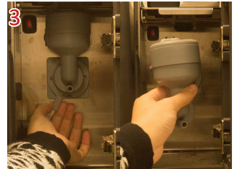
3 Unlock the mixer by turning the knob to the right. Take the mixer unit out.
