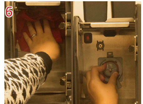
6 Wipe the powder module with a clean damp towel. Remount the knob and the ring back into the powder module pushing firmly until it clicks.
