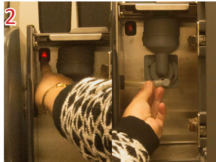
2 Press the power button to switch off the powder module. Pull out the tube connected to the mixer.
