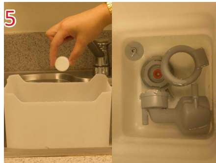
5 Dissolve an Egro Milk System Cleaning Tablet in a container with warm water. Place pieces of the mixer unit into the solution. Allow to soak for at least 1 hour.
