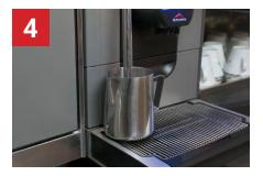
Reinsert the steam wand into the container with clean water and activate the steam wand again.
