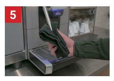
Remove the steam wand from the clean water. Wipe down the steam wand and activate the purge function. The steam wand is now ready for use.
