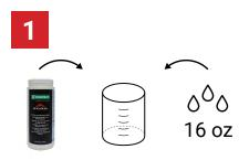
Prepare a cleaning solution by adding an Egro Milk System Cleaning Tablet to 16 oz of hot water.
