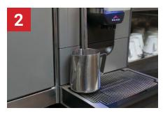
Insert steam wand into the solution and ensure that the nozzle is submerged. Activate the steam wand and let the solution react for at least 10 minutes.
