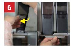
Make sure the dispensers are towards the middle into the mixer unit. Right powder hopper dispenser should be to the left. Left powder hopper dispenser should be to the right.
