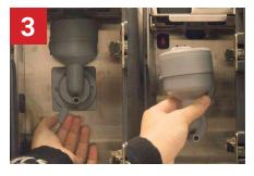
Unlock the mixer by turning the knob to the right. Take the mixer unit out.
