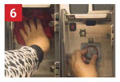
Wipe the powder module with a clean damp towel. Remount the knob and the ring back into the powder module pushing firmly until it clicks
