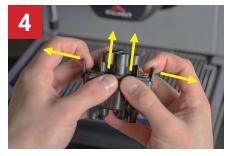
Seperate the brewing spout assembly by pushing out on the tabs while pushing up on the upper spout assembly. Soak the seperated spout assembly in the solution for at least 1 hour.
