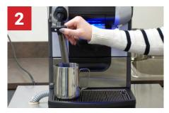
Activate the steam wand until the solution is heated and allow the wand to soak in the solution for 10 minutes.
