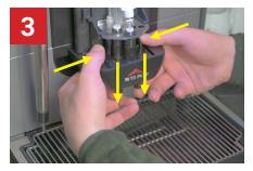
Push the tabs on the brewing spout assembly in and down to disconnect it from the machine.
