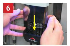
Slide the silver outlet cover down. The cleaning has been completed.
