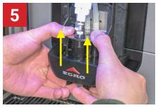
Reassemble the spout and reconnect it to the machine by pushing firmly upwards. Make sure all parts snap into place.
