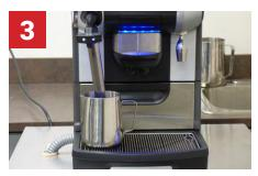
Dispose of the cleaning solution and refill with fresh water. Activate the steam wand until the water is heated.
