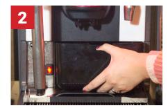
Open the front door, remove the bin, and dispose of the grounds. Wipe the grounds drawer clean, replace the bin, and close the front door. Confirm on-screen that you have emptied the grounds bin.
