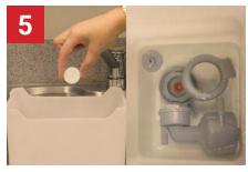
Dissolve an Egro Milk System Cleaning Tablet in a container with warm water. Place pieces of the mixer unit into the solution. Allow to soak for at least 1 hour.
