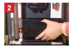
Open the front door, remove the bin, and dispose of the grounds. Wipe the grounds drawer clean, replace the bin, and close the front door. Confirm on-screen that you have emptied the grounds bin.
