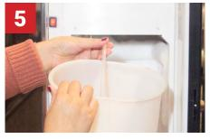
Place the container with the cleaning tablet in the refrigerator and insert the milk tube into the container. Tap "OK".
