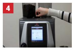
When prompted on-screen, insert one (1) Coffee Machine Cleaning Tablet into the chute on top of the machine.
