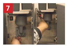
Reassemble the mixer unit into the powder module. Turn the knob to the left to lock. Reconnect tube to the mixer. Push power button to turn on the powder module.
