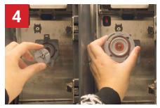
Pull out the mixer ring and the knob simultaneously.
