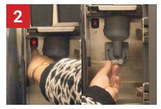
Press the power button to switch off the powder module. Pull out the tube connected to the mixer.
