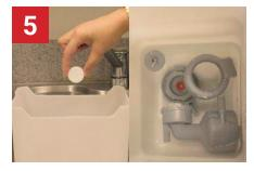
Dissolve an Egro Milk System Cleaning Tablet in a container with warm water. Place pieces of the mixer unit into the solution. Allow to soak for at least 1 hour.
