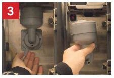
Unlock the mixer by turning the knob to the right. Take the mixer unit out.
