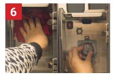
Wipe the powder module with a clean damp towel. Remount the knob and the ring back into the powder module pushing firmly until it clicks.
