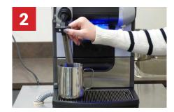
Activate the steam wand until the solution is heated and allow the wand to soak in the solution for 10 minutes.
